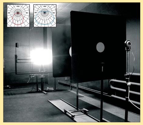
SEC is one of the few luminous technique producers that owns a PHOTOMETRIC LAB for measuring light parameters of lighting fixtures and lighting sources. Thanks to the 12m long goniophotometer we are able, even within the development process, to verify the photometric parameters of new lighting. All of this is done with special emphasis on harmony of design and optimal lighting parameters.
